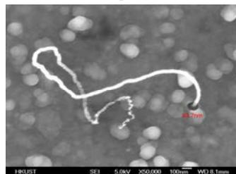
Figure 3: A single MWCNT grown through a via with diameter 93.7nm.
